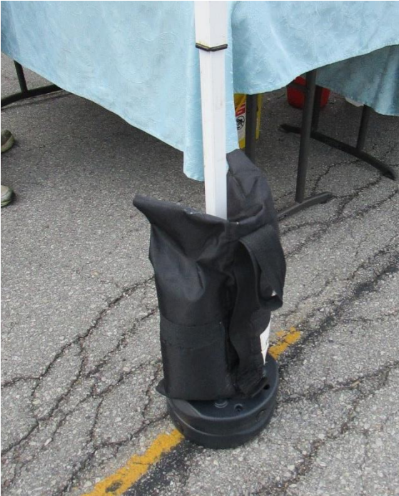
Canvas bags filled with rocks or sand. NOTE: These filled bags usually do not weigh 40 lbs each and must be doubled up (two weights per leg) or combined with other weights.
