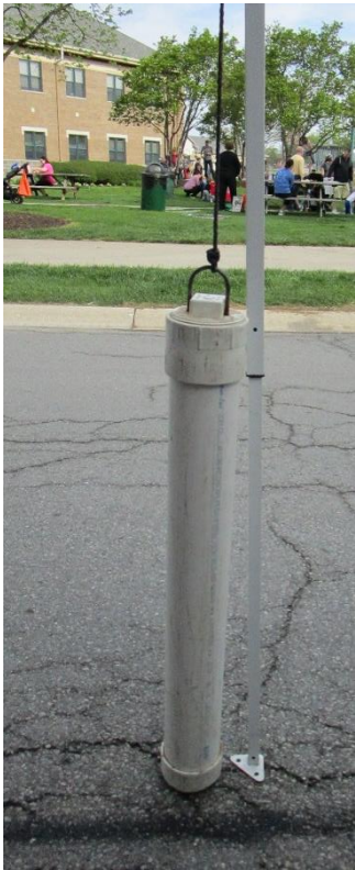
PVC pipe filled with cement and capped; must be secured in a way that it does not collide with customers or create a hazard.
