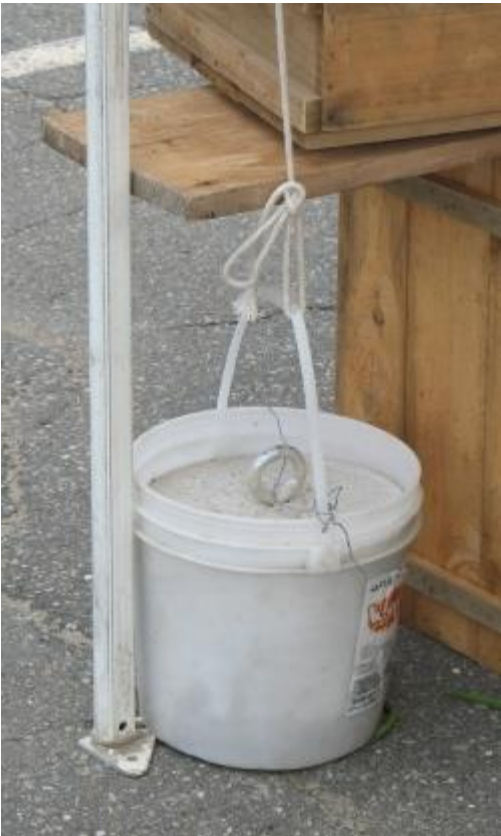
Bucket filled with cement and tied to each corner of the tent with a rope or bungee. It is NOT sufficient to place the can on the feet of the tent.
